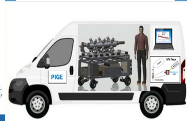
Figure S4: (Left) Centurion™ Mk1 system being loaded into a van for transport to an off-site demonstration >1000 miles away. (Right) The compact RFQ LINAC itself (shown assembled with Starfire's patent-pending RF power injectors) is approximately 4' long and can be modified for energies between 1–5 MeV.
