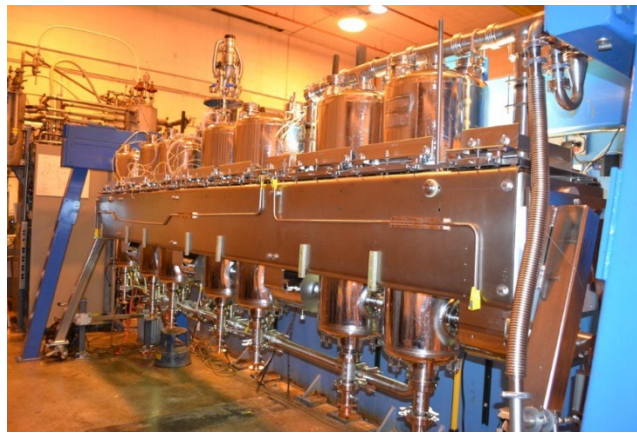
Figure 4.1: A string of superconducting cavities and focusing solenoids developed for a recent intensity upgrade of the ATLAS facility.
