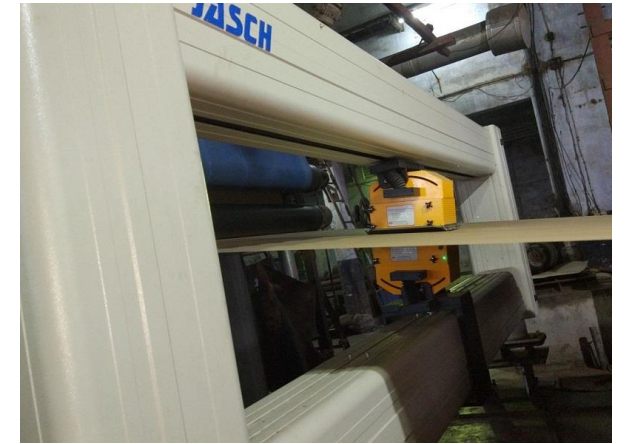
Paper/board weight using ^{85}\text{Kr} or ^{147}\text{Pm} (Beta-emitters) https://jasch.net.in/paper-global-trendsetting-technology
