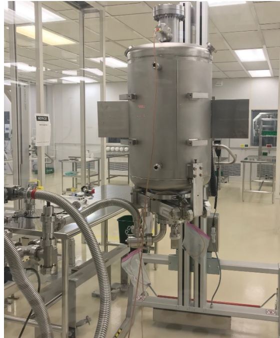
Cavity in He vessel
