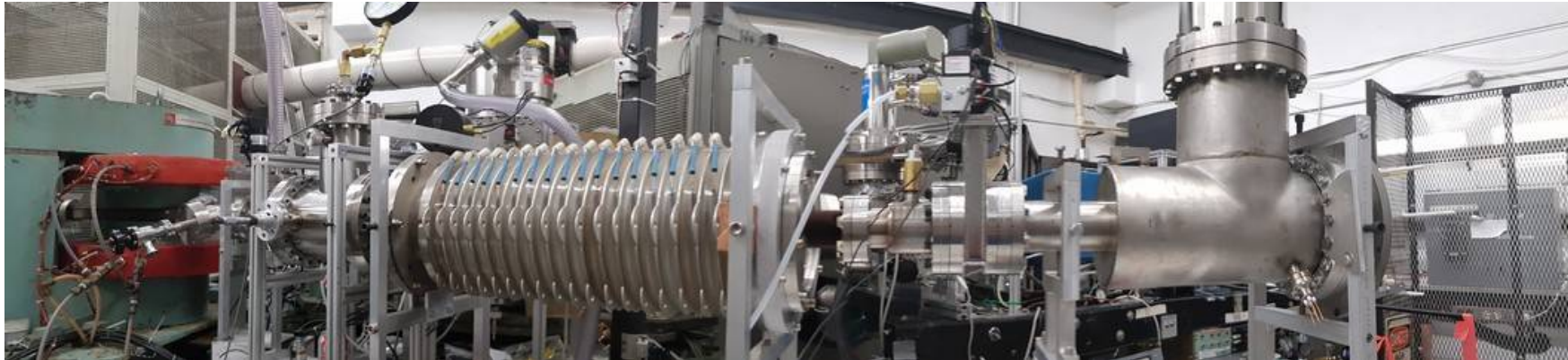
New, dedicated negative-ion injector at FSU Tandem-Linac
