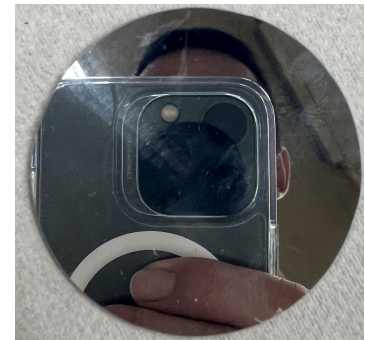
Surface roughness: 20 nm (ISO N1 polished surface)
