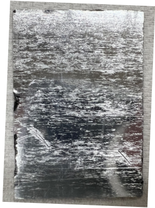
Surface roughness: 200 nm (ISO N4 polished surface)
